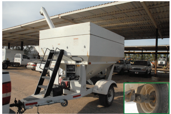
Figure 1. Examples of mobile scales used for load calibration of cotton (left) and grains (right) yield monitoring systems. Close up images in the bottom-right corners show weigh-bars load sensors installed in the 4 corners of the frame (cotton boll buggy) and at the wheels of the axle (grain cart).
