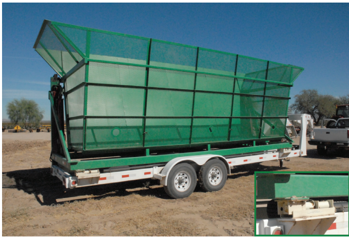
Figure 1. Examples of mobile scales used for load calibration of cotton (left) and grains (right) yield monitoring systems. Close up images in the bottom-right corners show weigh-bars load sensors installed in the 4 corners of the frame (cotton boll buggy) and at the wheels of the axle (grain cart).
