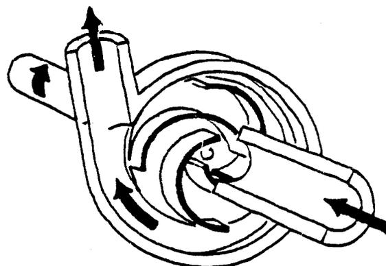
Figure 7.8 Centrifugal pump
