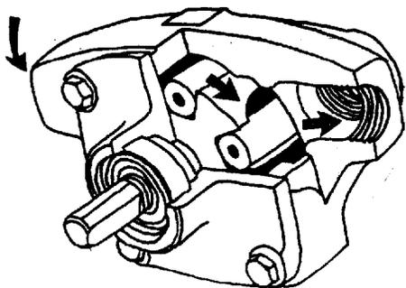
Figure 7.7 Roller impeller pump
