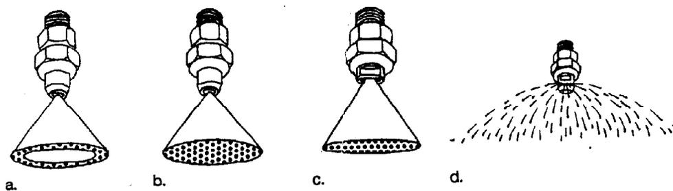
Figure 7.10 Nozzle types (a. hollow cone, b. solid cone, c. flat fan, d. flooding flat fan)
