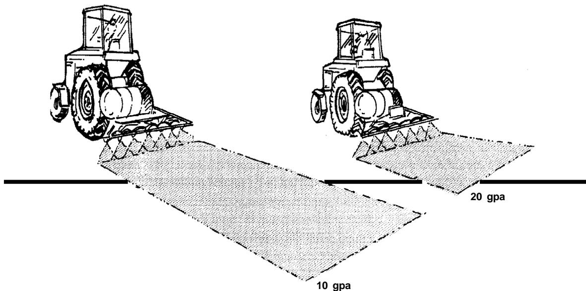
**Figure 6.1** Altering the volume applied by changing travel speed.
