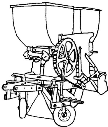
Figure 7.4 Granular spreader
