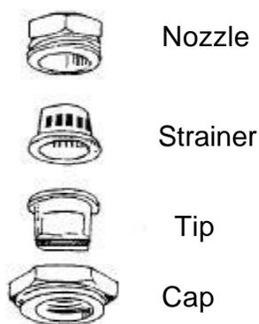
Figure 7.9 Parts of a nozzle
