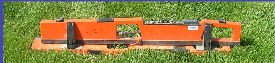
**Non-Destructive Electromagnetic Induction Conductivity Meter**
