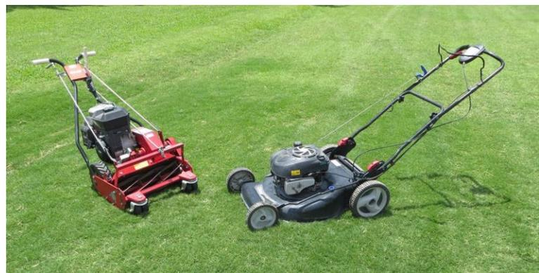
**Reel-type mower (left), and rotary mower (right)**
